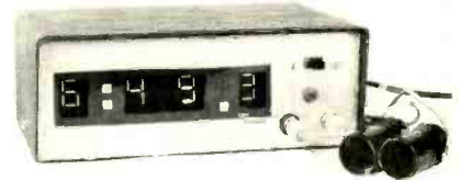
ELECTRONIC STOPWATCH uses modular construction to make it easy to duplicate. Measures time intervals from 0.1 second to 9 minutes 59.9 seconds. ....see page 39
