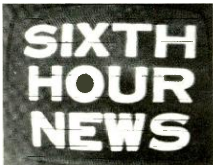
FIG. 1—IGNITION INTERFERENCE or other pulse-type signals may produce short, sharp lines or dashes. Increasing the received signal strength or shielding lead ins may help.
